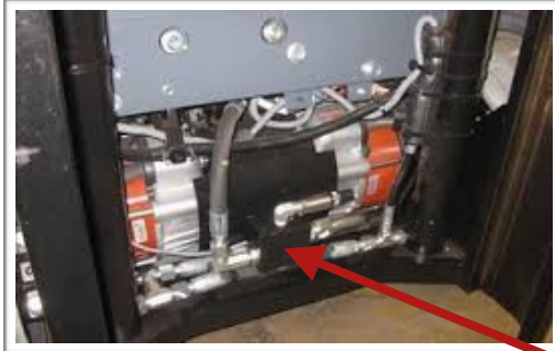
Pressure transducer installation in hydraulic block divider
