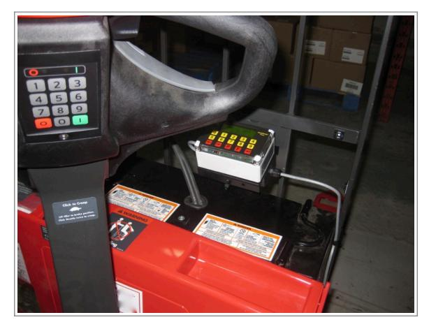
The **OSC2-EP** is a simple comprehensive unit designed to provide single electric pallet truck or small fleet with the ability to monitor impacts and control that only certified operators are allowed access to the lift trucks and ensure that prior to shift use a safety check is done.
