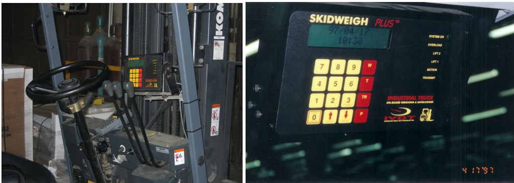
Example of the pressure transducer installation / digital indicator on Toyota forklifts with short mast
